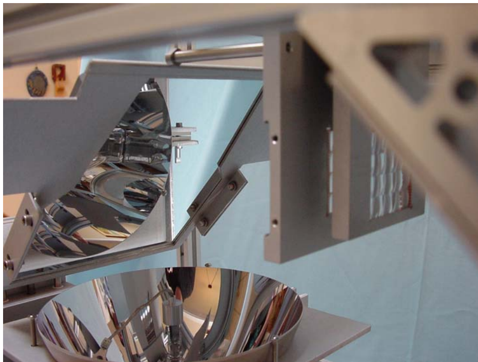
The “optical engine” of Sun 2000 Solar Simulators
